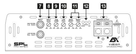
There are two RCA inputs on the **LINE INPUT**, each of which is controlled in mono. The input **LOW VOLTAGE** is suitable for low level signals from 0.4 to 3.6 volts. At the input **HIGH VOLTAGE** you can connect a high level signal from 1.0 to 9.0 volts, such as that provided by a DSP.
