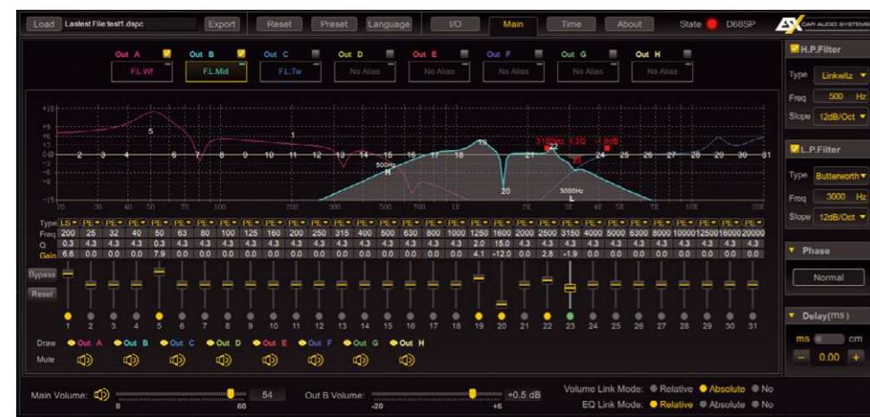
Equalizers and crossovers are set on the main screen. Master and channel levels are available. Absolute or relative linking of channels is possible here
