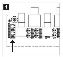
First disconnect the device from the power supply. Then remove the housing cover and locate the six jumpers on the circuit board. These are located to the left of the audio inputs.
