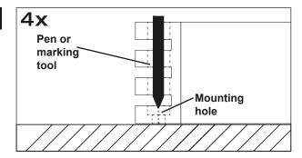
Keep the amplifier at the chosen mounting location in the vehicle. Then mark the four drill holes with an appropriate pen or marking tool through the designated mounting holes at the amplifier.
